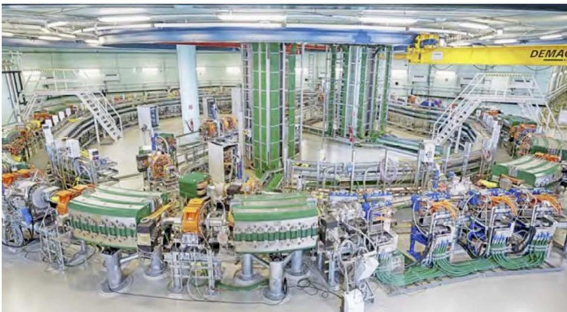
**Figure 5** - The MedAustron synchrotron feeds 1 proton treatment room with gantry, 2 heavy ions treatment rooms with 3 beams (2 horizontal and 1 vertical), and 1 experimental room.
