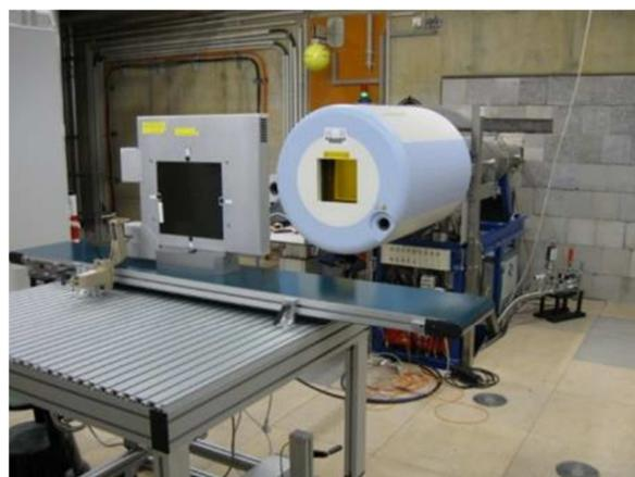
*Figure 17 - Nozzle and sample positioning system at the HIT facility.*
