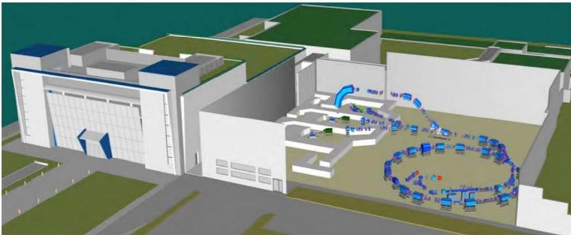
**Figure 4** - Perspective view of the CNAO, which features 3 treatment rooms with 4 therapeutic beams (3 horizontal and 1 vertical), and 1 experimental room (not represented).
