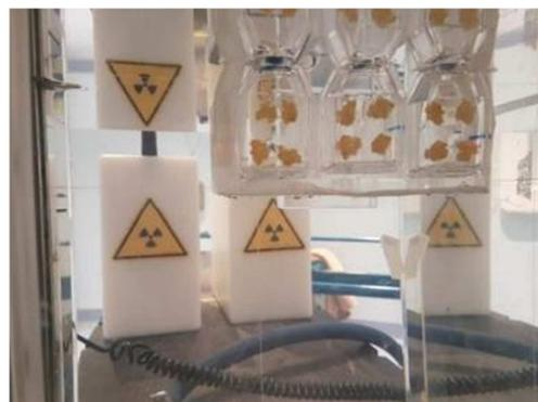
*Figure 13 – Example of in vitro irradiation set up at CNAO.*
